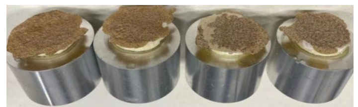
ADHESION TESTING SHOWING SUBSTRATE FAILURE
